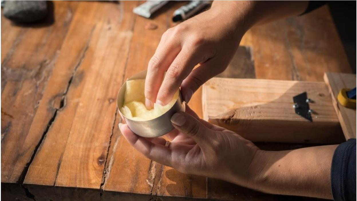
Cut a square of fiberglass insulation and insert it into the stove base piece. This acts as a wick for the alcohol fuel.
