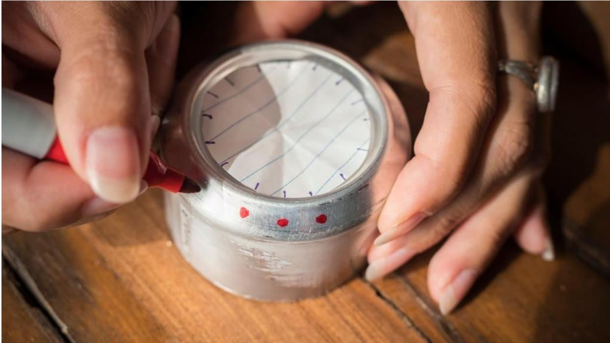
Turn one can upside down, and place a piece of paper on it. Trace a circle on the paper using the bottom of the can as a guide. Cut out the circle and fold it in half four times. Unfold and place on the bottom of the can. Use a marker to dot the can at each fold; there should be 16 evenly spaced marks. Drill each dot using a 1/16" drill bit.
