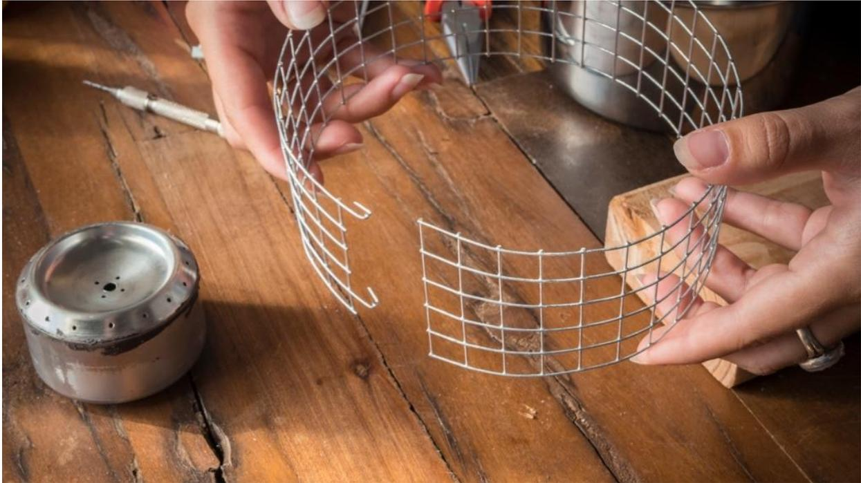
Using wire cutters, clip a piece of metal mesh to 2.5" tall and 17" long. On one short side, clip off all but two of the metal threads. Bend the remaining two into hooks. Clip off any extra threads. Form the mesh into a circle, and secure the hooks to stabilize. Place your cooking pot on top and adjust the stand size if necessary.
