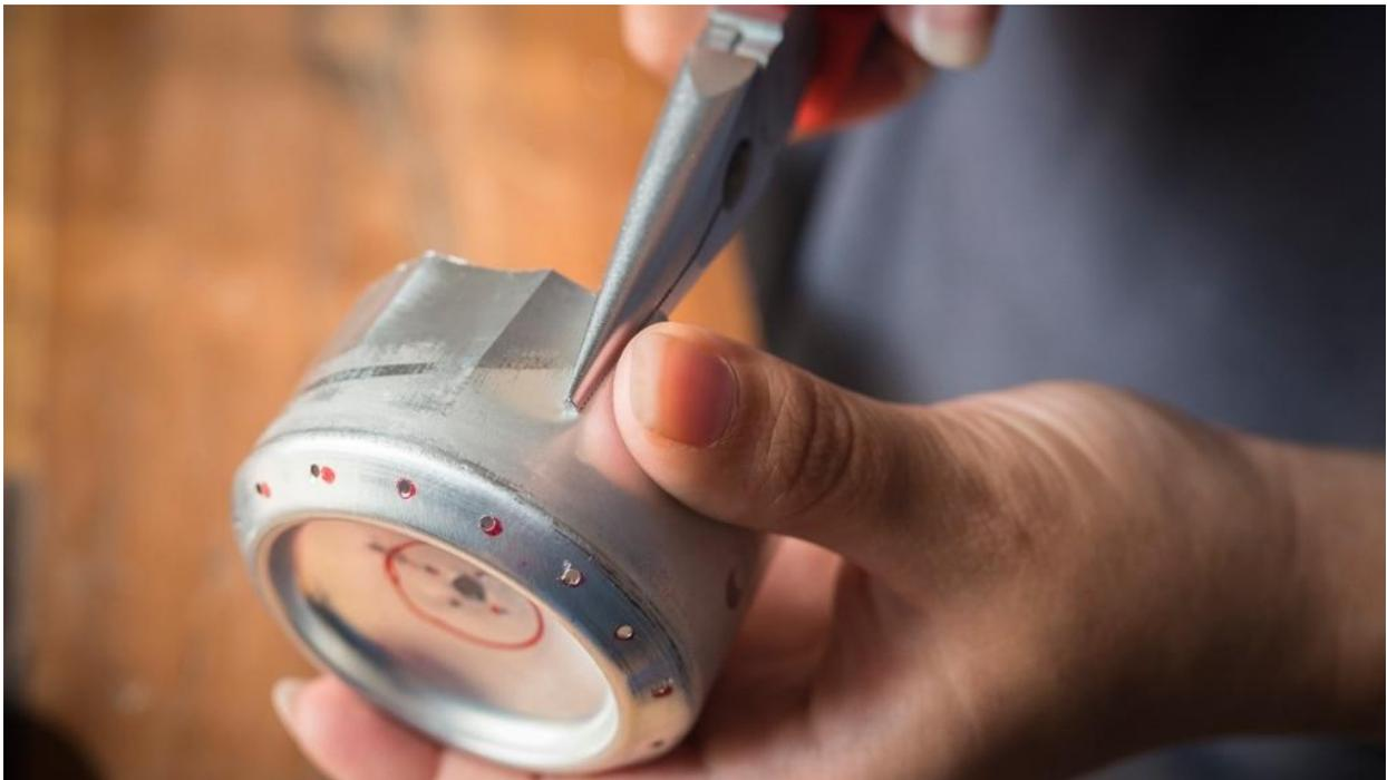
Prepare the two stove pieces to slide together more easily. Crimp all the way around the opening of the top piece with pliers. Use a different, full beverage can or similar object to work around the inside edge of the base piece to stretch it slightly.
