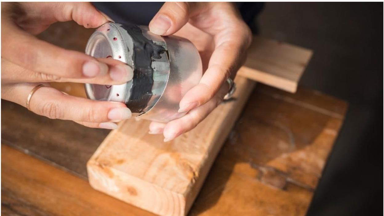
Mix up some high heat epoxy per the instructions and apply it to the outside of the crimped edge of the top piece. Carefully slide the top into the base piece, pressing evenly and firmly. Wipe off any excess epoxy and allow to cure per the package instructions. Sand off any remaining dried epoxy.
